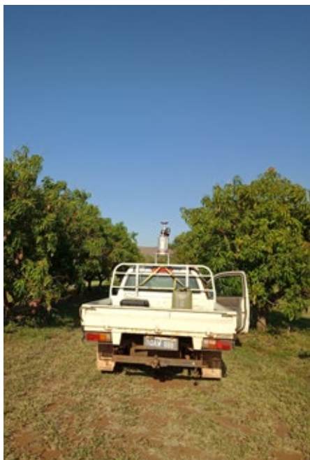
LiDAR scanner mounted on back of ute © Liqi Han
