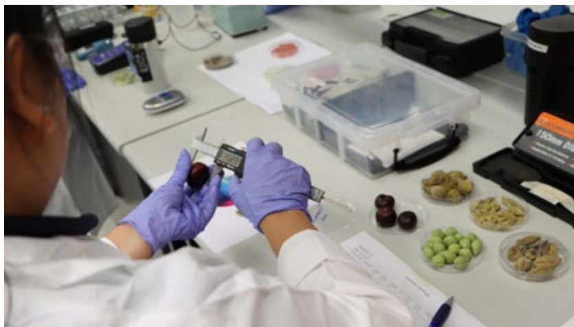
Dr Anh Phan demonstrates use of callipers to measure fruit to seed ratio – equipment included in the chemistry toolkit, Coopers Plains Lab, June 2021. Pic: UQ
